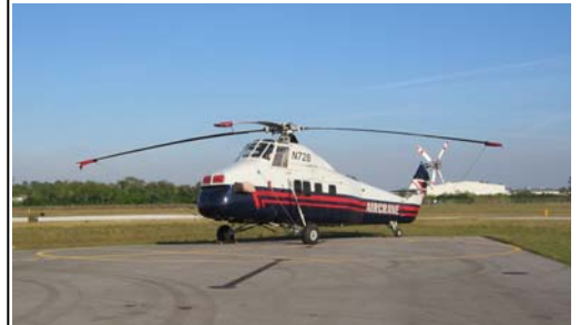
Sikorsky S-58T N72B was in Fort Myers recently lifting air conditioning equipment on several construction projects.
