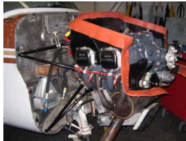
Newly overhauled engine on N5158Q
